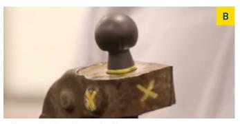
Ball joint stud in a damaged steering knuckle.
