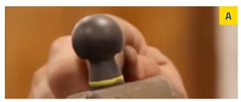
Ball joint stud in an undamaged steering knuckle.
